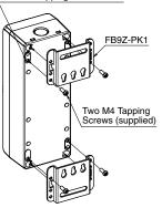
Attach the FB9Z-PK1 on the FB series with the supplied screws (two M4 tapping screws).
