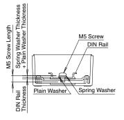
Mounting Switches/Pilot Lights on DIN Rail
