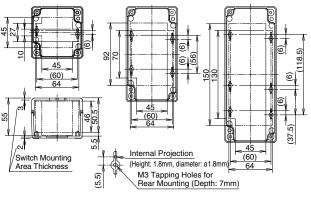
Choose an enclosure in consideration of switch's depth behind the panel and the mounting centers of the adjacent switches.
